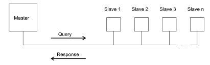
In the MODBUS Protocol the master can address individual slaves, or, using a special "Broadcast" address, can initiate a broadcast message to all slaves. The Integra Digital meter do not support the broadcast address.
