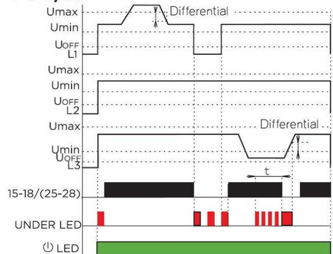
The time delay and differential trip levels help to prevent relay chatter as the monitored voltage level varies.
