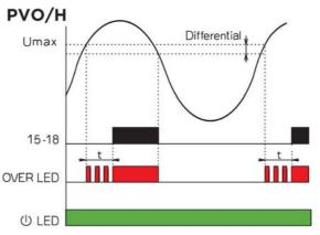
The time delay and differential trip levels help to prevent relay chatter as the monitored voltage level varies.
