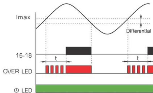
The time delay and differential trip levels help to prevent relay chatter as the monitored current level varies. As the relays have changeover contacts, the relay outputs can be inverted by wiring to the alternative terminals 15-16 or 25-26.
