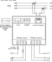
Please note for 3P3W configuration L2 is connected through the neutral and not V2.
