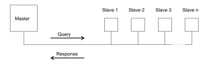
In the MODBUS Protocol the master can address individual slaves, or, using a special "Broadcast" address, can initiate a broadcast message to all slaves. The Paladin Advantage Transducer does not support the broadcast address.
