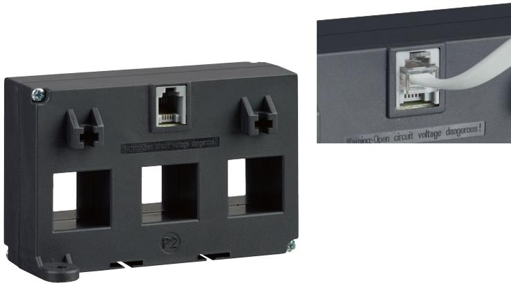
The 3-in-1 current transformer range are for use with the INTEGRA 1221 digital metering system which combines three traditional current transformers in one moulding case with a RJ12 connection and 1.5m cable included for simple and easy error free installation. Available with 25, 35, 45 and 70mm centers.
